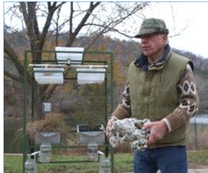
J. David demonstrating the relationship between land use, surface water and groundwater with the use of his "rain machine."
